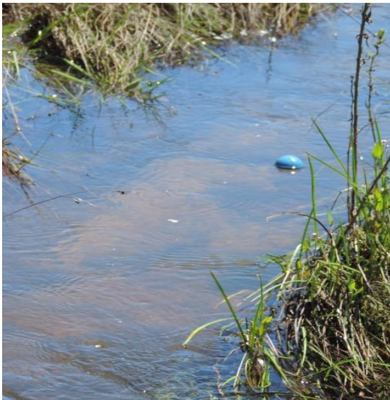
Fig.6. Squash ball measuring flow speed
